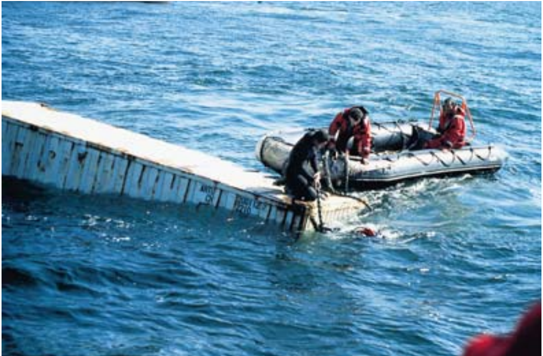
A diver fitting a hoisting sling around a container (photo Cedre).
