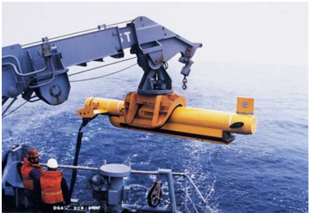
Towed side-scan sonar DUBM42 being lowered into the water (photo : DGA France).
