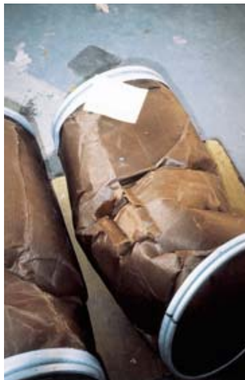
Kraft drum after spending 48 hours at a pressure of 20 bars (photo Cedre).
