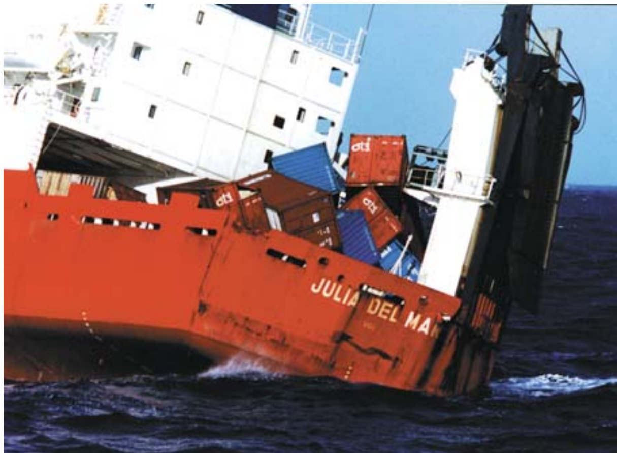
The poorly-secured cargo of Julia del Mar - 1989 (photo SAVR: Service Audiovisuel Régional).
