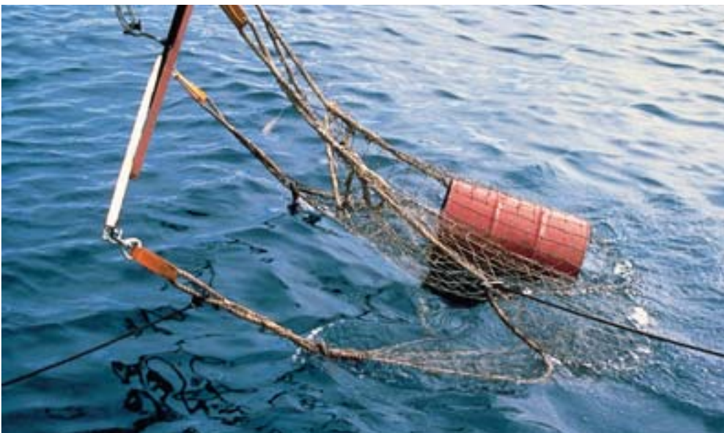
Specially designed trawler net for the recovery of drums (photo Cedre).
